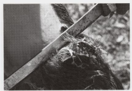
Close-up of wet-scraping: note the patch of grain, with hair still attached, being puked off in front of the blade
